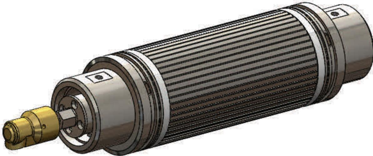
FIGURE 4—Feed Roll Assembly
