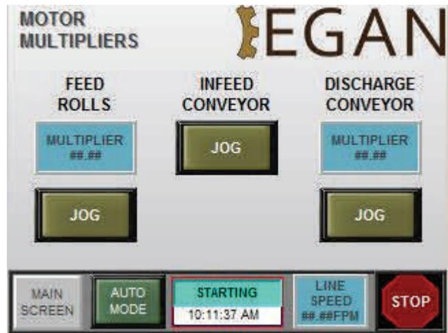
This is the MOTOR CONFIGURATION SCREEN. Here, the user is able adjust the multiplier (value is a multiple of the line speed setting) and also jog the motors for manual control.
