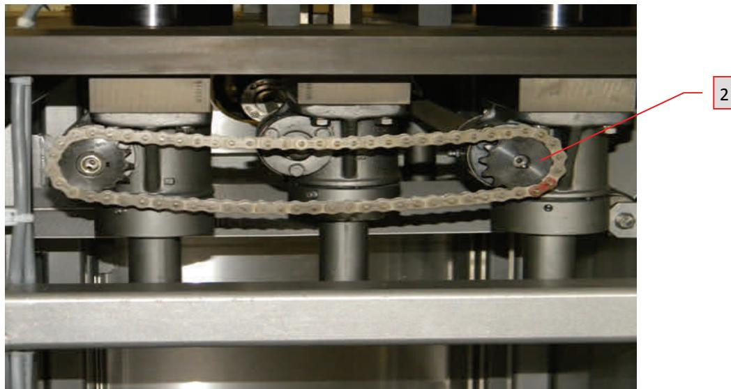
FIGURE 11—Detail of Jack Screw Mechanism in Cabinet
