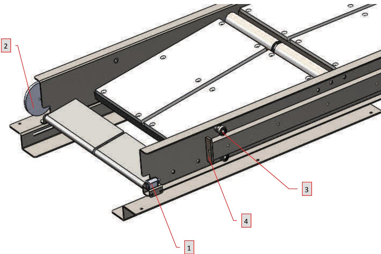
FIGURE 18—retracting Conveyor Assembly with Side Plates Removed
