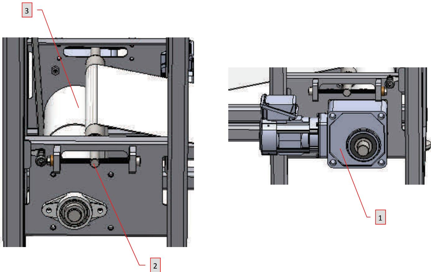
FIGURE 20—Discharge Conveyor Drive Assembly
