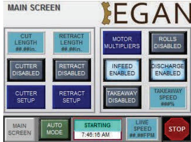
This is the HOME SCREEN. Here, the user is able adjust settings, enable and disable specific components, and navigate to other setup screens.
