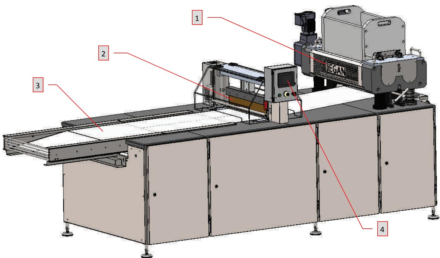
FIGURE 1—BAR CUTTER AND RETRACT CONVEYOR
