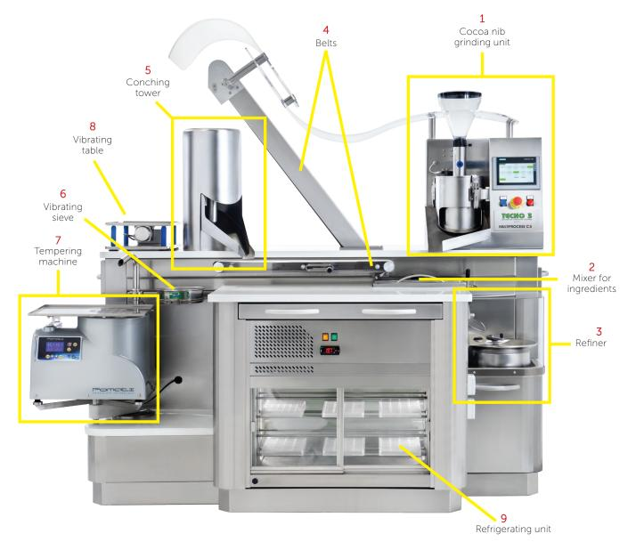
After the mixing stage, the outlet connecting to the refiner is opened: the product flows down due to the effect of gravity and the refining stage starts. The product comes out on a tilted conveyor belt that leads it to the upper part inside the cylindrical conching tower.
